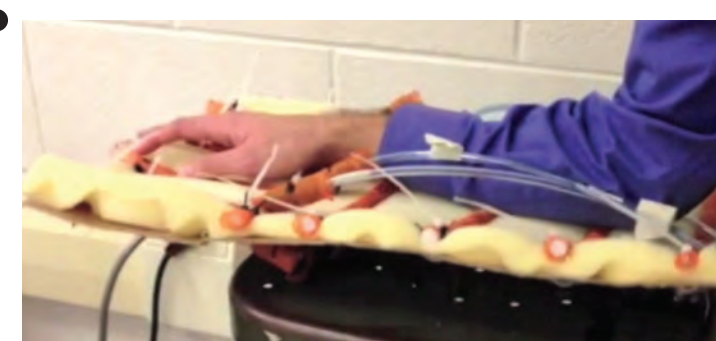
A continuum-robotic 2D surface actuated by McKibben, pneumatic muscles.
